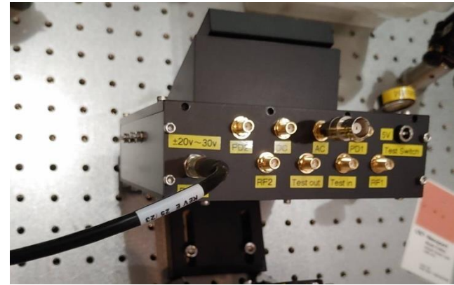
kHz BHD: Balanced Homodyne Detector for detection below 100 kHz.
