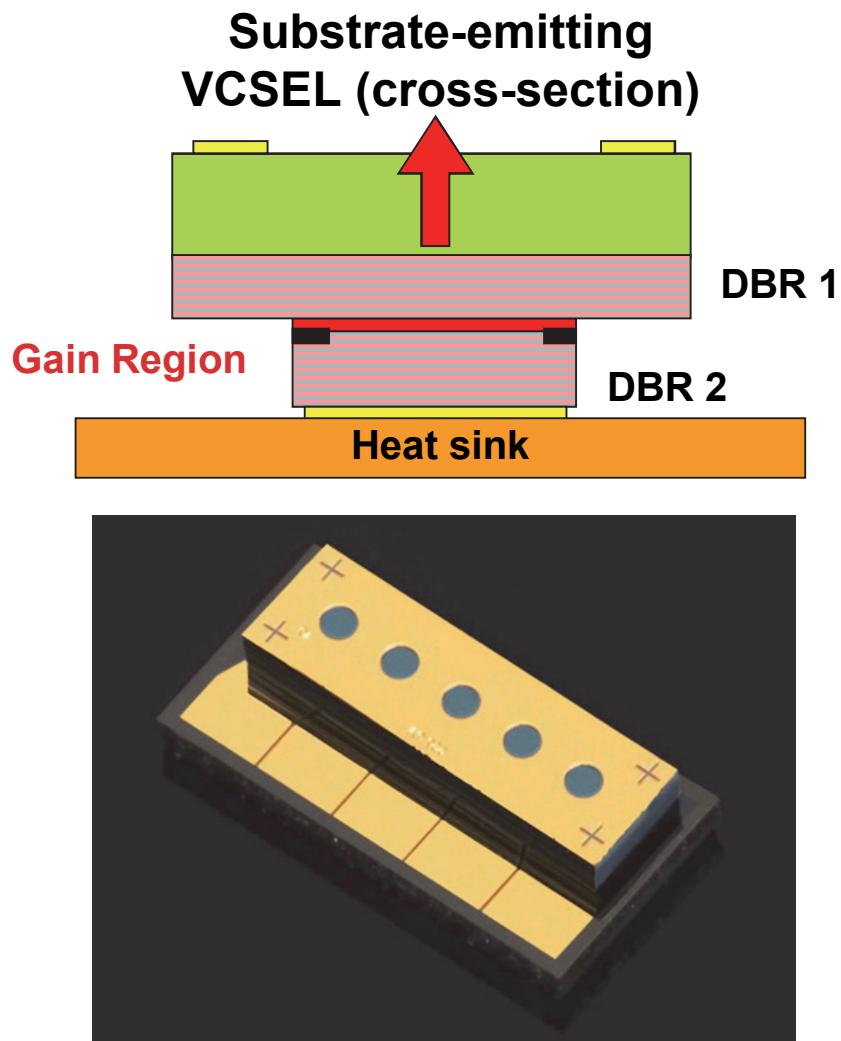
Large-aperture linear VCSEL array, Aerius Photonics, LLC (FLIR Electro-Optical Components)
