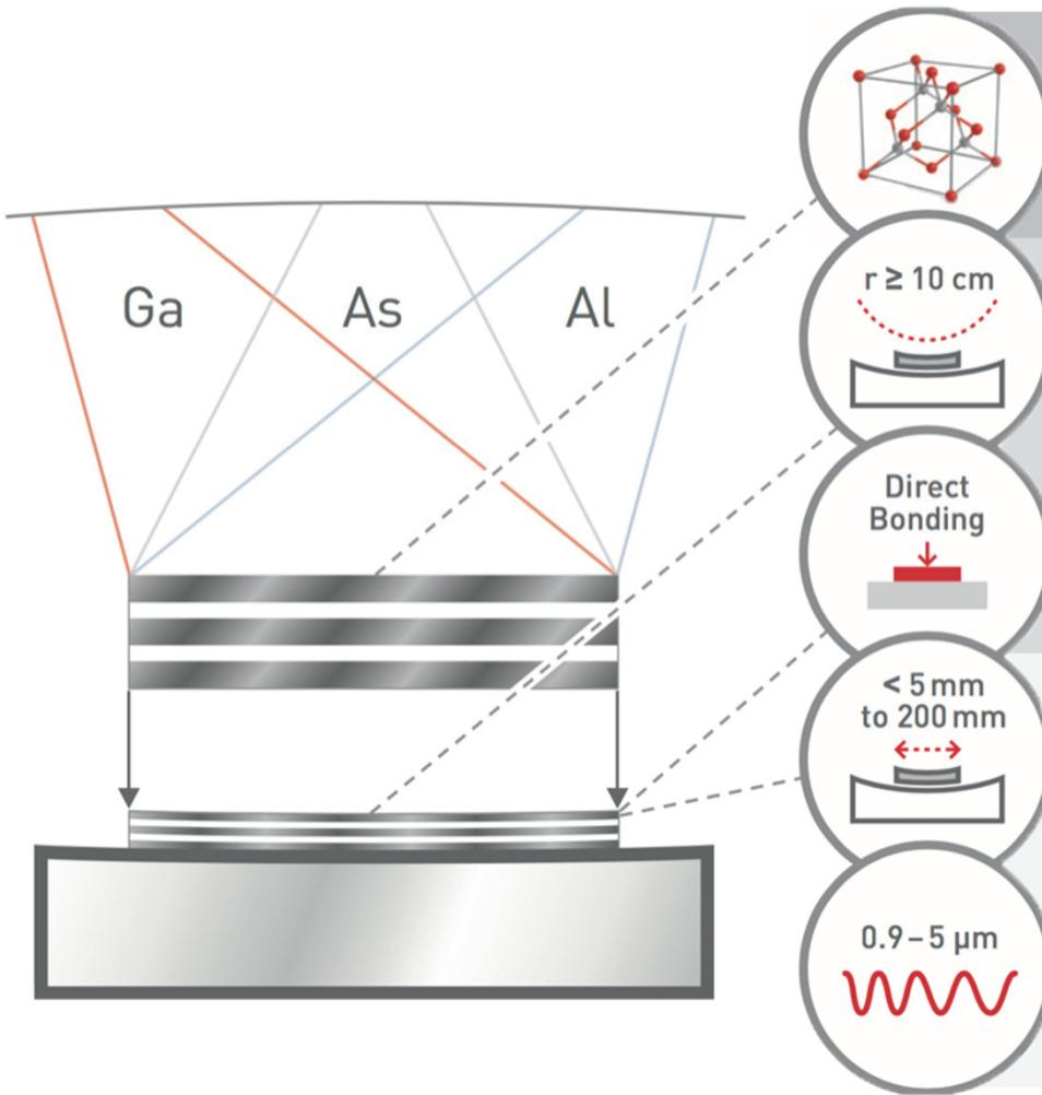
Monocrystalline GaAs/AlGaAs heterostructures grown on GaAs wafers by molecular beam epitaxy
