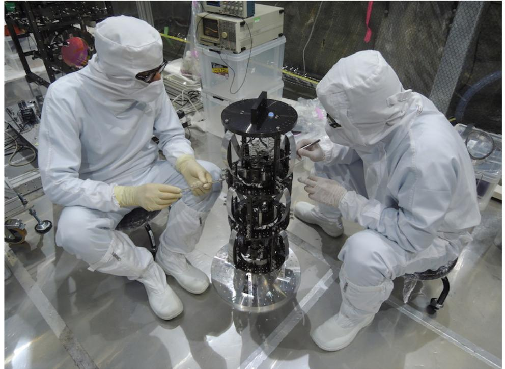
All the HLVISs in total have been installed into each cryostat.
