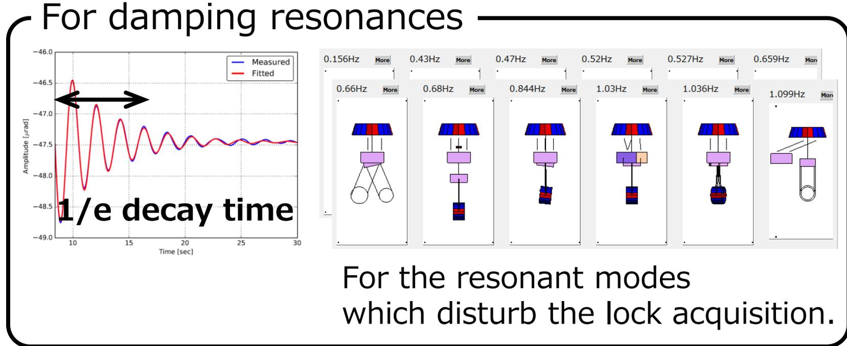
→ We have to measure the decay time constants w/ and w/o damping controls, in order to verify the damping control performance, FOR ALL THE TYPE-A/B/Bp SUSPENSIONS.
