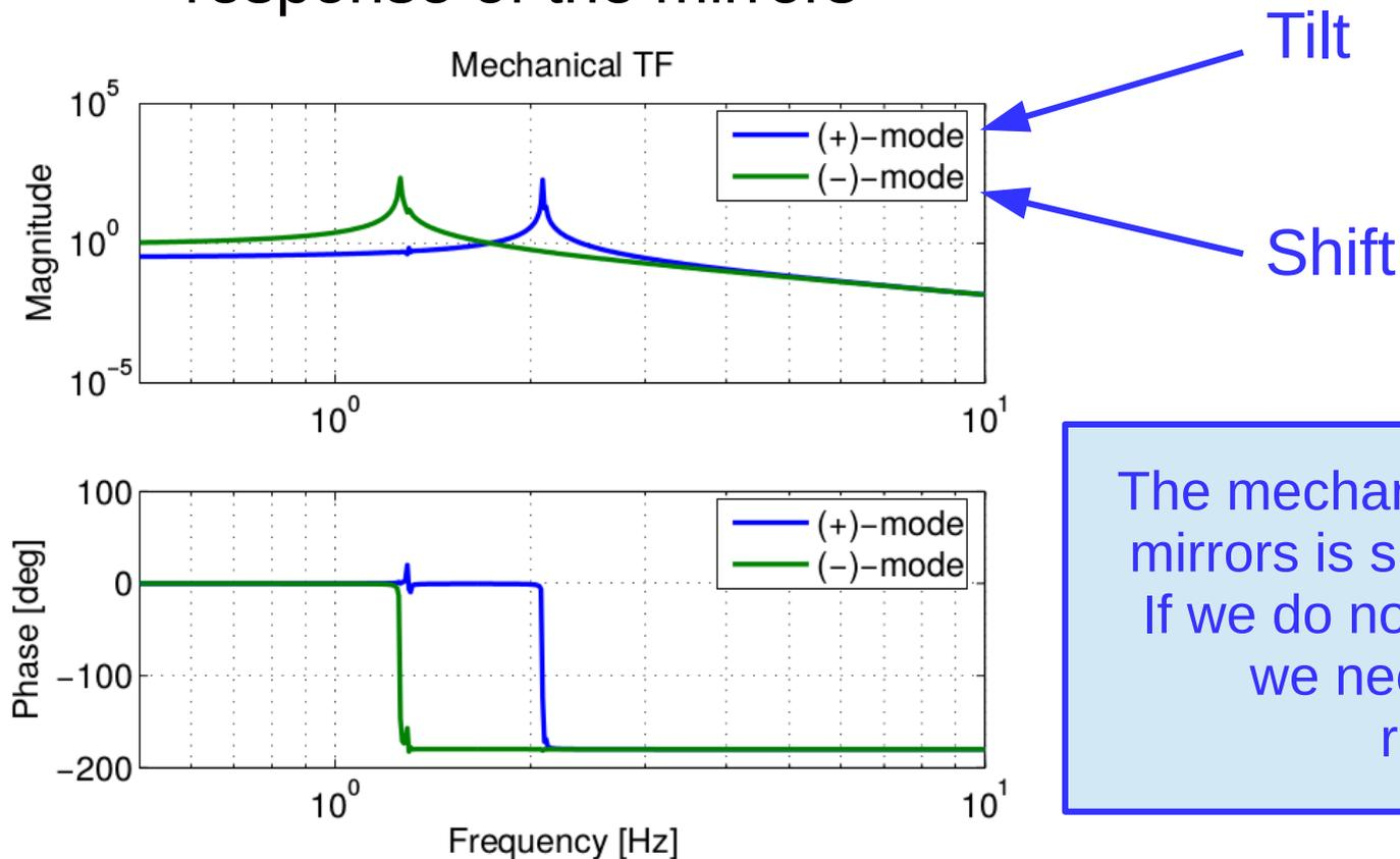
The mechanical resonance of the mirrors is shifted in frequency → If we do not decouple both dofs we need to deal with 2 resonances
