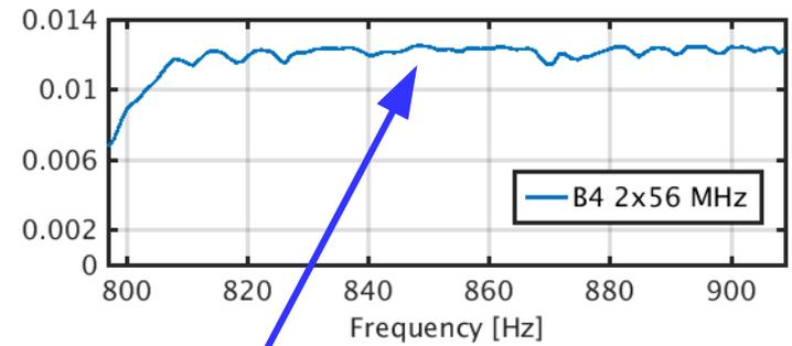
*Once the alignment is engaged the sidebands power stabilizes*
