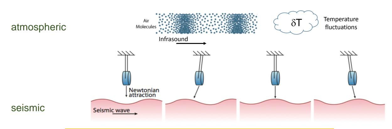
Gravitational coupling between the mirrors and surrounding mass density fluctuations
