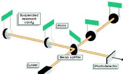
The frequency range of Virgo extends from 10 to 6,000 Hz. This range as well as the very high sensitivity should allow detection of gravitational radiation produced by supernovae and coalescence of binary systems in the milky way and in outer galaxies, for instance from the Virgo cluster.
