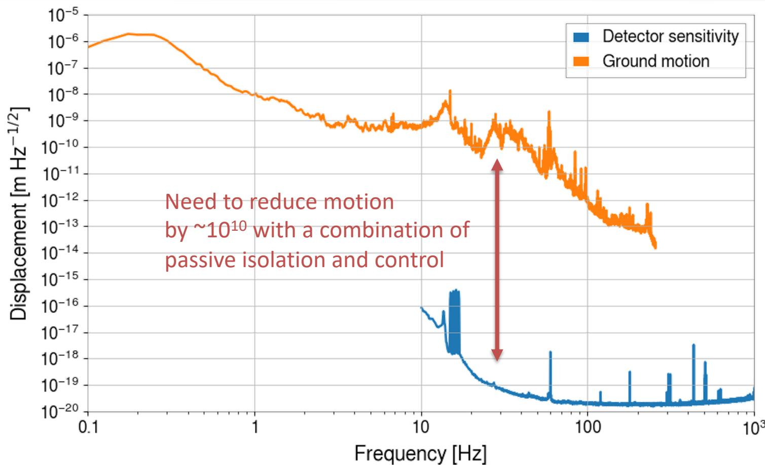
Compensate for **1-10  $\mu\text{m}$  of motion below  $\sim 1 \text{ Hz}$** , without introducing spurious displacement larger than  $\sim 10^{-19} \text{ m/VHz}$  above  $\sim 10 \text{ Hz}$
