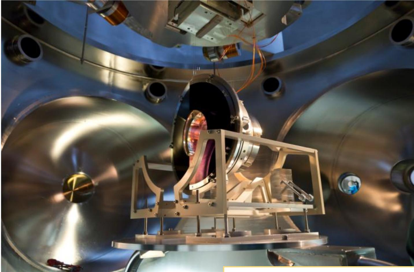
*IMC end mirror payload in MC tower*
