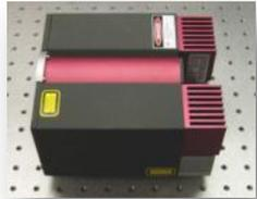
**Commercial NPRO Nd:YAG Laser from coherent (P=1 W @1064nm)**
