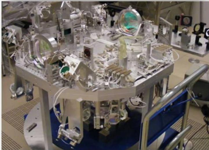
→ Ultra high vacuum compatible optical bench used to inject the Laser beam in the Virgo Interferometer. Used also to pre-stabilize the laser frequency (a rigid reference cavity (RFC) is below this bench)
