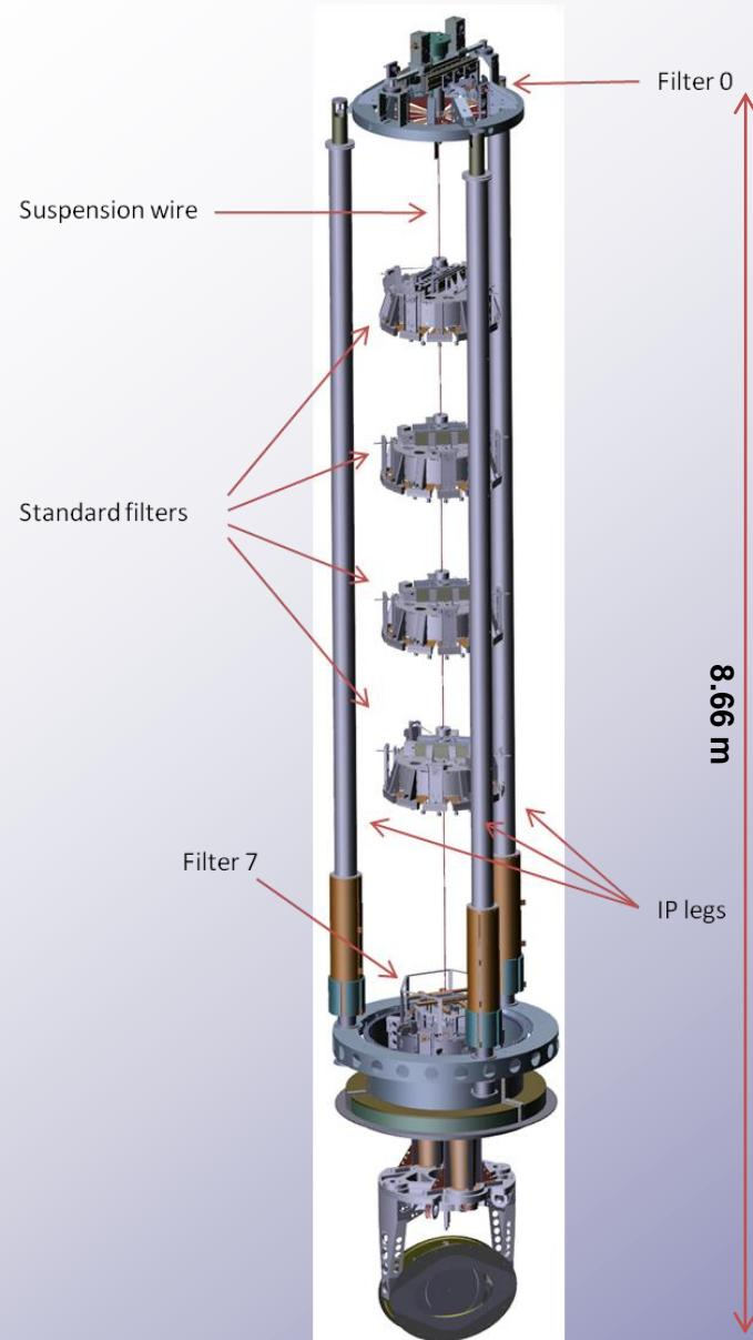
The AdVirgo superattenuator (SA) is a complex mechanical device capable of providing more than **10 orders of magnitude of passive seismic isolation in all six degrees of freedom above a few Hz**
