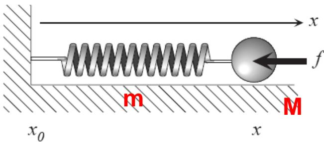
$$H_X = \frac{\omega_0^2(1 + i\phi) + \frac{m}{M}\omega^2}{\omega_0^2(1 + i\phi) - \omega^2 + i\frac{\gamma}{M}\omega}$$
