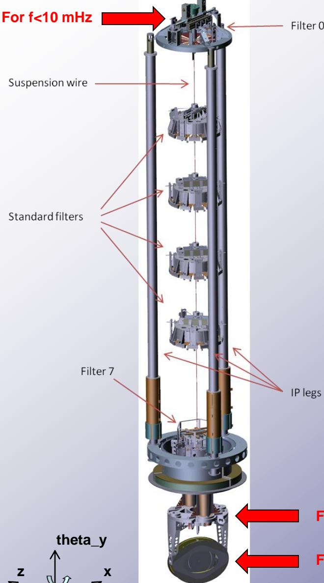
The control system has been designed using a hierarchical strategy regulated by the dynamic range of the actuators.
