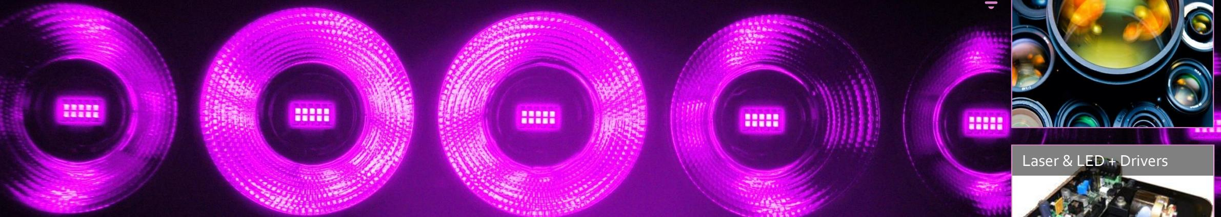
All in-House designed LED illuminators for 300km/h automatic track inspection
