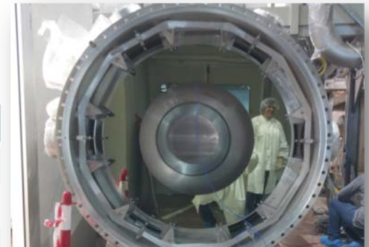
AR-coated (R<0.5%) metallic baffle
