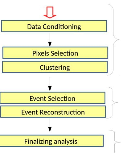
Data conditioning (removing frequency lines and whitening procedure)  $\rightarrow$  FFT of the data data (single interferometer)
