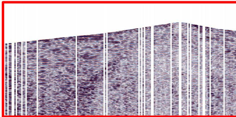
Velocity analysis, stacking, gain functions, FX deconvolution and trace mixing
