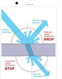
The Bidirectional Scattering Distribution Function (BSDF) is used to characterize scattering as a function of the angular position of the incident and scattered beams. [units of steradian<sup>-1</sup>]
