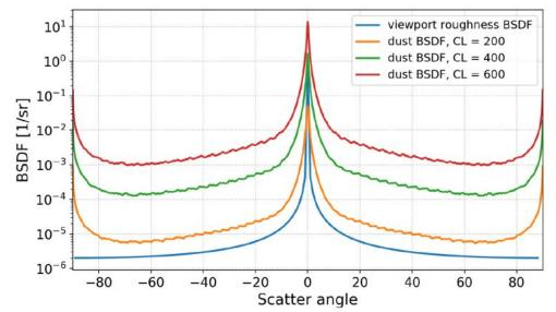
Viewport used in AdV O3 for FIS: 0.3nm surface roughness (TIS = 12ppm) CL=200 (i.e. 1 particle> 200um in 0.1m<sup>2</sup>, for a steep particle distribution ie s=-0.927) corresponds to (in horizontal orientation):
