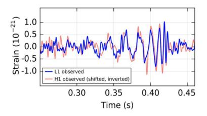
The wave holds for less than a second. We see a few cycles. The quantity on the Y-axis is the strain of the space: the variation of the distance over the arm of the instrument. It means that the arms (which are 4 km long) are stretched of the order of 10<sup>-18</sup> m. An incredibly small quantity. However, the signal is pretty clear.
