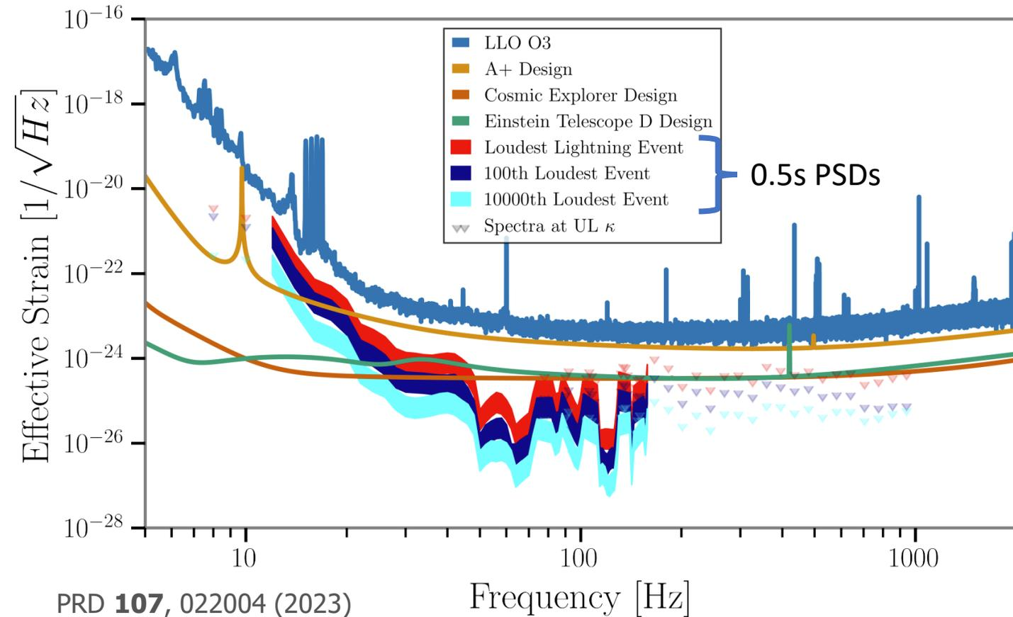
Schumann resonances as well as a large number of EM-provoked transients would be visible in ET-LF without improved payload design.
