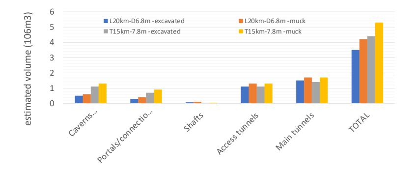
The volume of excavated and crushed material was obtained by multiplying by a factor of 1.2 the volume of the rock in place, in order to take into account the voids in the pile.
