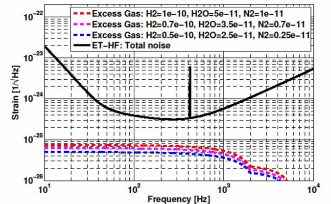
Figure 6.16: Phase noise given by the residual gases compared to the expected sensitivity, computed for the appropriate beam profile for different gas compositions. (Goal gas composition: Hydrogen [ $1 \cdot 10^{-10}$  mbar], Water [ $5 \cdot 10^{-11}$  mbar], Nitrogen [ $1 \cdot 10^{-11}$  mbar])
