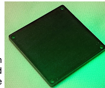
Diamond-like carbon (DLC) coated stainless steel sample
