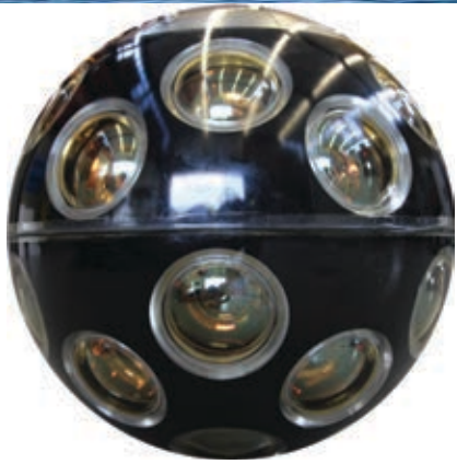
Digital Optical Module (DOM) A fly's eye light detector Inside a 17" glass sphere
