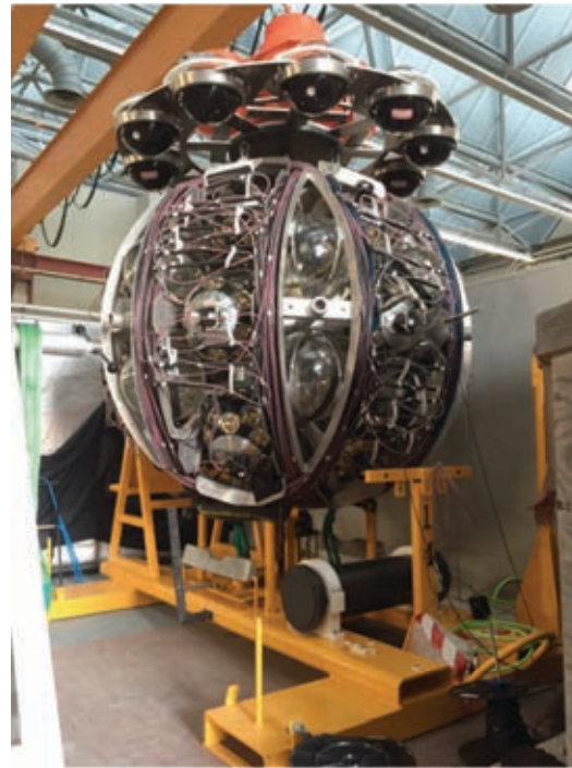
Detection Unit a vertical string with 18 DOMs
