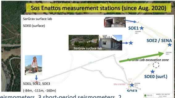
4 broadband seismometers, 3 short-period seismometers, 2 magnetometers, 1 microphone+microbarometer and 1 tiltmeter distributed over underground and surface stations
