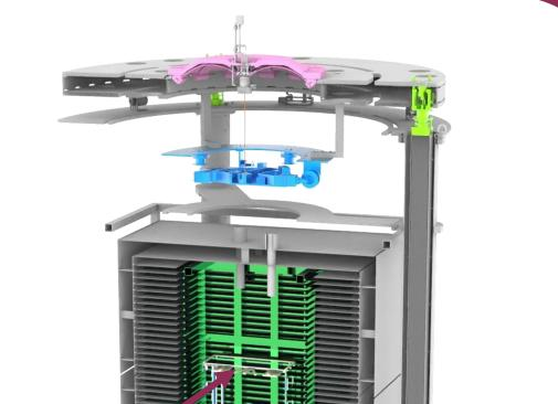
• The sensors close to the mirror must be capable of operating in harsh cryogenic environments with extremely high sensitivity to monitor the residual vibration at the last isolation stage.
