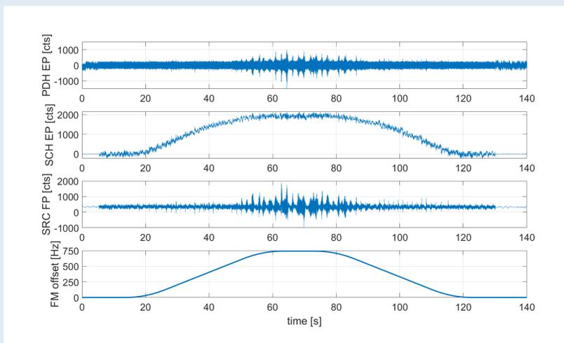
Fig.6: The plot shows the time series of different signals when the SRC was detuned from 0Hz to 750Hz and back using the new locking scheme. At the time  $\sim 5.5$ s, the error signal employed to control the SRC was switched from the one obtained with the Schnupp technique to the new PDH error signal. The frequency of the SCL was then ramped by actuating on the FM input of the PLLs LO. The out-of-loop Schnupp EP shows that the SRC was actually detuned.
