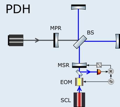
Fig.4: With the new method, a frequency-shifted auxiliary laser, the sub-carrier laser (SCL), is injected through the dark port of the IFO. The error signal for the SRC locking is obtained using the PDH technique [4].
