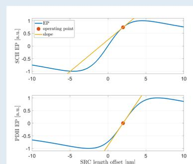
Fig.8: When the SRC is detuned, the operating point of the new error signal is kept at the zero-crossing value, and the slope is always the same. If the Schnupp error signal is used instead, one must add an offset to the EP and adjust the gain.
