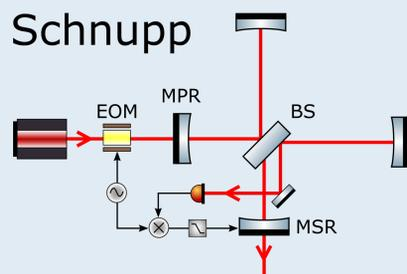
Fig.3: The Schnupp technique [3] is based on the phase modulation at the input of the interferometer. The error signal for the SRC longitudinal control is obtained after demodulation from the PD located in one of the AR ports of the BS.
