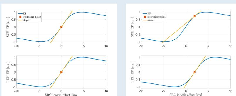
Fig.7: The two error signals look the same when the SRC is tuned...
