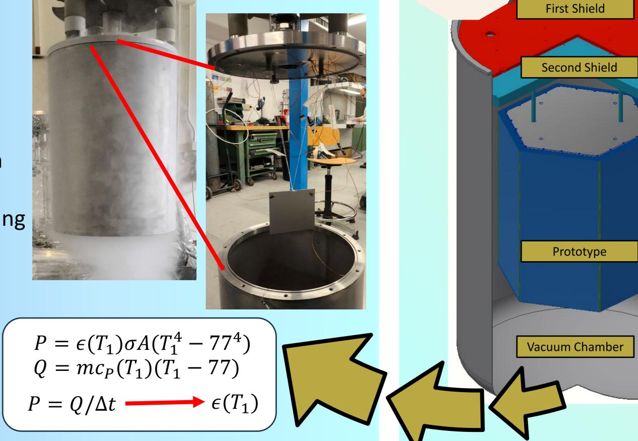
2. ROMOLO: downscaled version of OTS. A suspended hexagonal based structure (thickness 6 mm) with adjusted rods anchored by means of insulating bolts, implementing 15 layers of aluminum foil and cooled down by pulse tubes in a cryostat. This test focuses not only on the effectiveness of the isolation of the RML, but also on the feasibility, the ease of installation and the structural integrity.
