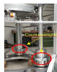
Fig. 8: The counterweights are mounted on the IP legs
