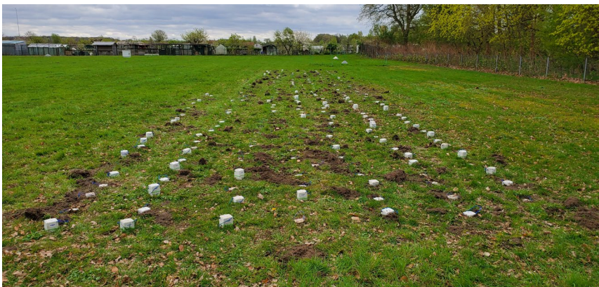
400 3C 5Hz SmartSolo Geophones getting calibrated at KNMI site
