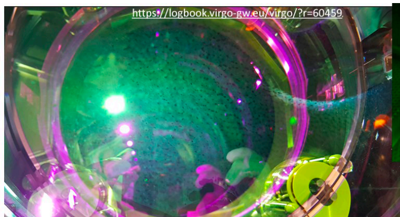
Figure 13: Surface of the old NE mirror before its removal from the vacuum tank in June 2023
