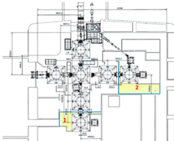
Figure 50 - Current clean areas (ISO6 / Class 1000) could be extended like in the picture. The blue lines are the potential expansion of the new cleanrooms, serving new chambers of DET and INJ, with a rationalized entrance: separate for personnel and for materials. PRM2, SRM2 and SPRB could have a portable clean room or light structure support with clean air box.
