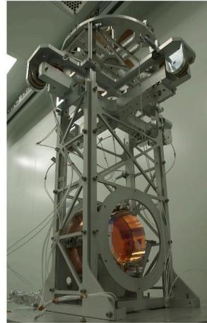
*Figure 37 - Block scheme and picture of the Adv+ Filter Cavity payload from which the benchtop double pendulum suspensions are derived.*
