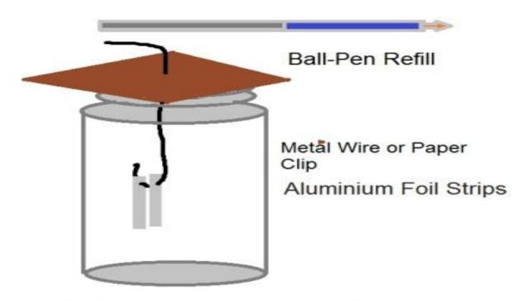
A simple electroscope to detect a charged body
