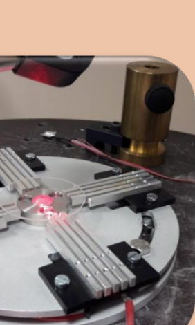
Internal view of the vacuum chamber. The sample is placed on a hemispherical support and excited via adjacent electrodes for mechanical loss measurements.
