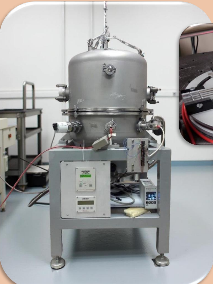
Vacuum chamber housing the GeNS system for mechanical loss measurements.
