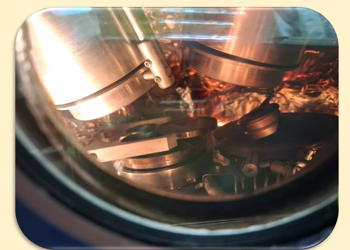
View through the viewport showing the inside of the RF sputtering vacuum chamber.
