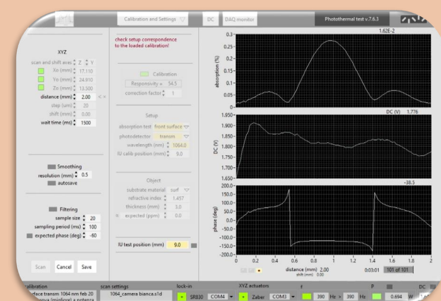
LabVIEW-based graphical user interface (GUI) developed for real-time control and data acquisition in PCI measurements.
