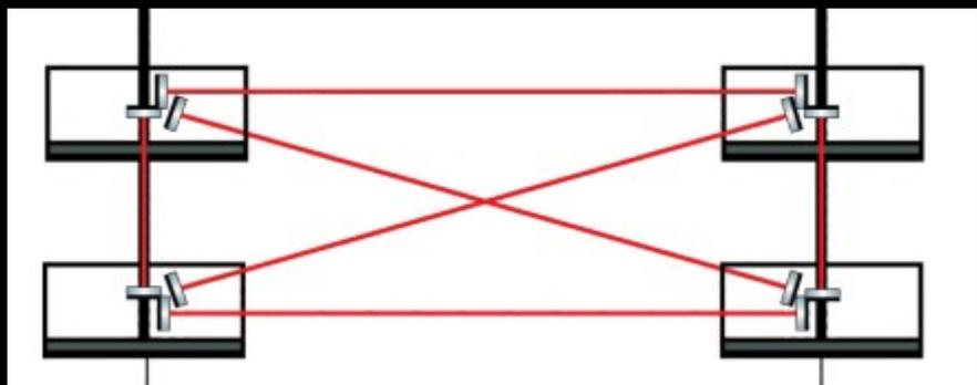
Optical Rigid Body concept using a network of interferometric cavities between stage-0 and stage-1 of both suspended platforms
