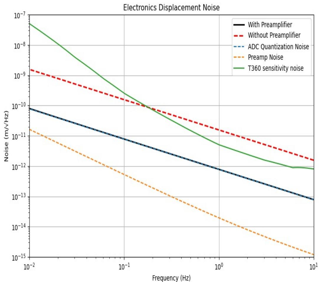
a) Electronics displacement noise
