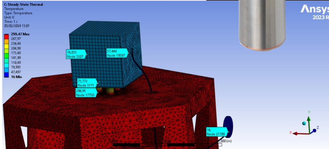
Thermal link design: Minimizing the length of the flexible braided copper section is essential
