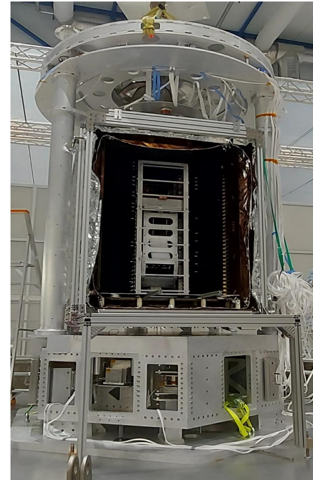
After integration of outer cryostat including LN 2 shield and GHe panels
