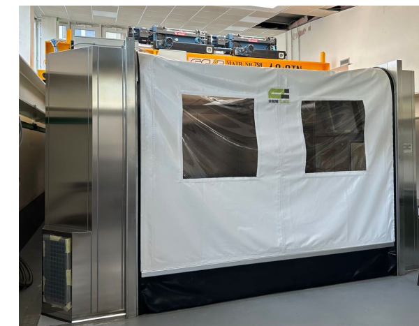
Clean Booth for Payload ops. ISO 6 at rest (ISO 7 under operations)
