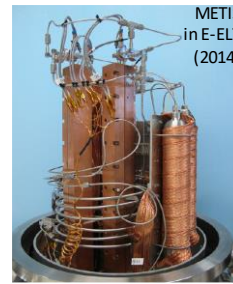
Long-life vibration-free 4.5 K sorption cooler for space applications, J.F. Burger (2007)
