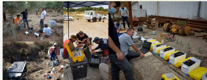
Deployment of seismic stations at the ET candidate site in Sardinia Credits: Luca Naticchioni
